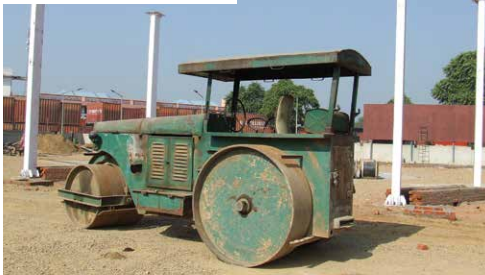
A Britannia-Road-Master motor roller manufactured by the Britannia Engineering Co. Ltd pauses during use at a new construction site adjacent to the main NH8 road about 60 miles south of Delhi.
