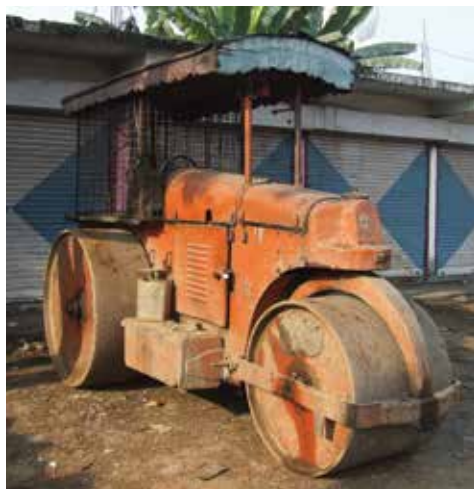
A motor roller built by Jessop & Co. Ltd in India under licence from Aveling-Barford Ltd, England. It was one of two which were parked close to the bazaar in Siliguri. A plate on the roller indicated that it was sold and serviced by Greaves Cotton & Co. Ltd of Bombay, Madras & Delhi.
