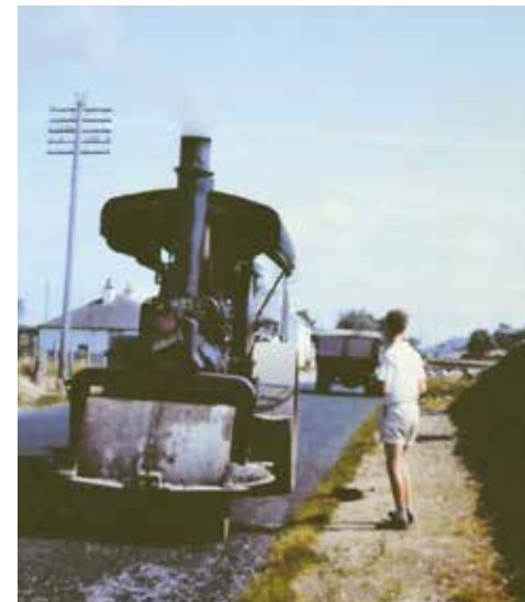
Another view of Fowler No.16402. Note the 'chimney extension' to improve the draft. These two images were taken on 6th July 1964. Norris Forrest
