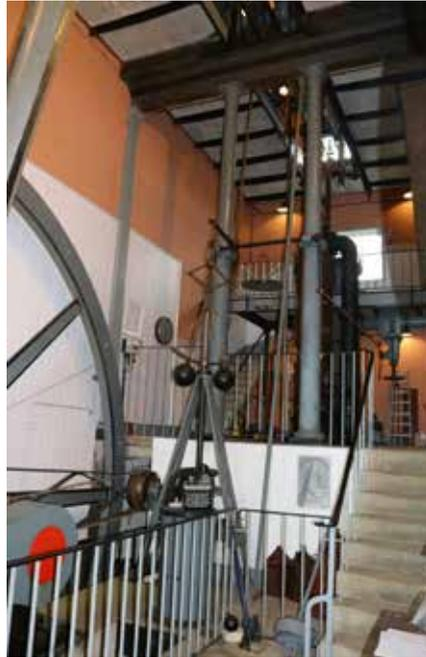
*The impressive beam engine at Stretham. It can be turned by an electric motor.*
