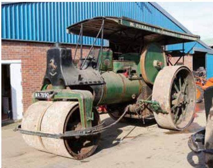
*A&P R15 No.3586 of 1895 is a mighty engine, listed at 15 tons weight but no doubt more when in working condition. Note the tyres are held on with wooden wedges.*
