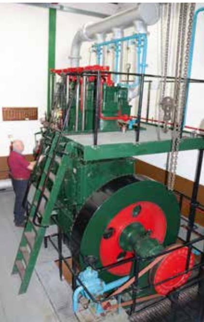
*Another engine which was run was this three cylinder Allen of Bedford diesel, moved here from another pumping station.*
