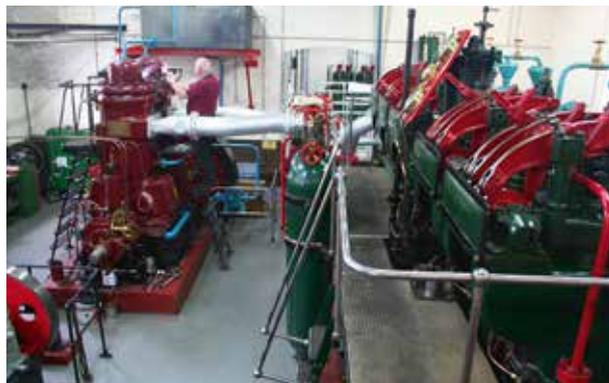
*The Vickers Petter hot bulb engine on the left is started by powerful twin blowlamps. On the right is another Mirreles diesel, this time a five cylinder one.*
