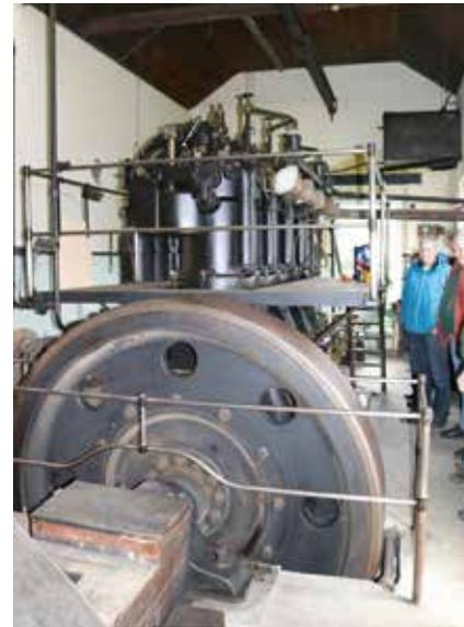
*Stretham also has an air blast Mirrlees Bickerton & Day four cylinder diesel engine installed in 1925.*
