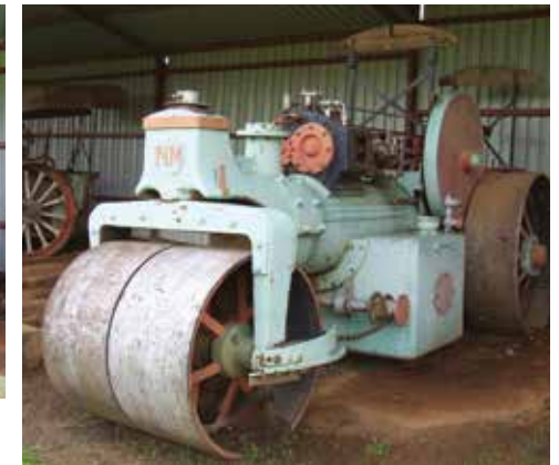
Aveling No.5396, unusually fitted with a large belly tank and one of a trio of similar rollers – designated as a 'Special Road Roller' – and the first of a trio of identical 12 ton rollers supplied to 'Crown Agents for the Colonies' on 25th November 1903, destined for Pretoria in South Africa!
