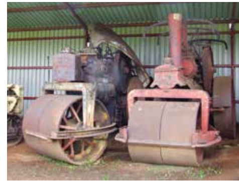
Fowler No.15546 on the left with a very non-Fowler like forecarriage head with No.16667 to its right. The former roller and others at Sandstone showed considerable damage which appeared to have been caused by poor handling at some time in the past.
