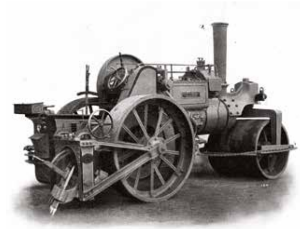
The Morrison Patent design of scarifier as fitted to a 10-12 ton Aveling slide valve compound roller.
