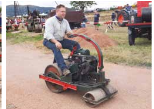
Rolling the chippings with the Motor Units roller.
