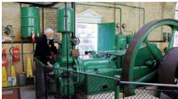
Bob Barnes starts one of the Campbell engines. It is started by compressed air.
