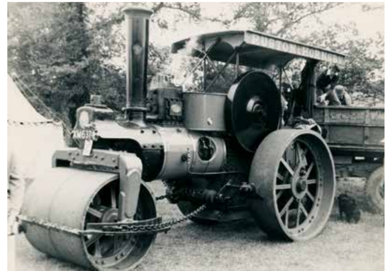
John Brice's 1922 Ruston & Hornsby SR Class No.115123. Note the repairs to the front forks done a long time ago.
