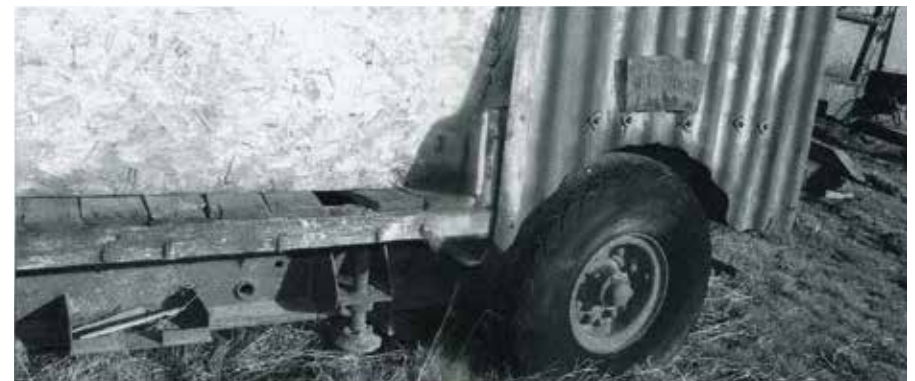
One of the levelling jacks still in situ.
