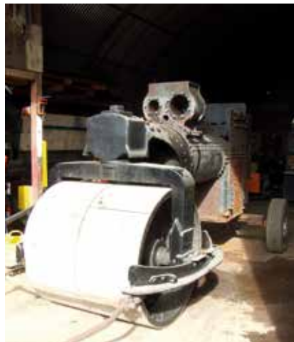
The front end of the roller with the cylinder now bolted in position.
