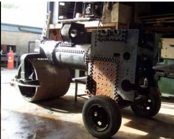
This shows the roller on its 'carrying wheels', fabricated in order to make for ease of moving it around.
