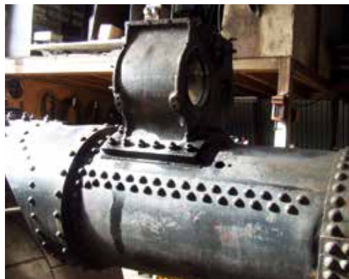
Another view of the all-important cylinder in position on the boiler barrel.
