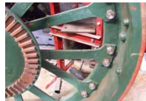
Having turned the roll around, the new bolt heads are very noticeable.
