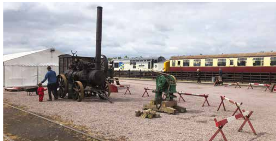
Simon Tansley & Ed Crane's 1928 Marshall S type 6nhp portable, driving the small stone crusher.
